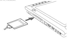
Figure 2-5. Installing a PC Card
